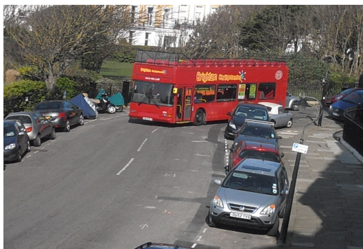
Photo 4: Bus swings wide into opposite lane at pedestrian access gate.
